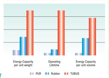
**ACE TUBUS profile dampers** are high performance damping elements made from a special Co-Polyester Elastomer. They have a high energy absorbing capacity compared with other materials.
