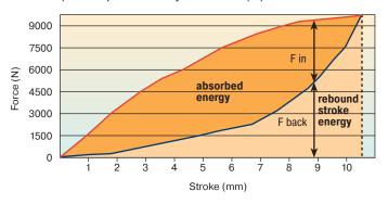
With the aid of the characteristic curves above you can estimate the proportion of the total energy that will be absorbed. Example: With the impact energy of 50 Nm the Energy-Stroke diagram shows that a stroke of about 8.8 mm is needed. On the Force-Stroke diagram you can estimate the proportion of absorbed energy to rebound energy at this stroke length.
