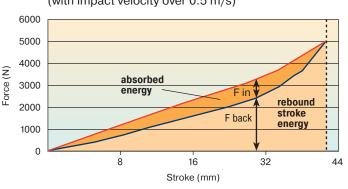
With the aid of the characteristic curves above you can estimate the proportion of the total energy that will be absorbed. Example: With impact energy of 50 Nm the Energy-Stroke diagram shows that a stroke of about 31 mm is needed. On the Force-Stroke diagram you can estimate the proportion of absorbed energy to rebound energy at this stroke length.
