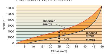
With the aid of the characteristic curves above you can estimate the proportion of the total energy that will be absorbed. Example: With impact energy of 50 Nm the Energy-Stroke diagram shows that a stroke of about 25 mm is needed. On the Force-Stroke diagram you can estimate the proportion of absorbed energy to rebound energy at this stroke length.
