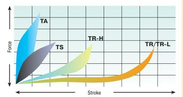
Characteristics of dynamic energy absorption for impact velocity over 0.5 m/s. For impact velocities under 0.5 m/s, please request a static characteristic curve.
