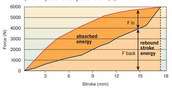
With the aid of the characteristic curves above you can estimate the proportion of the total energy that will be absorbed. Example: With impact energy of 50 Nm the Energy-Stroke diagram shows that a stroke of about 14 mm is needed. On the Force-Stroke diagram you can estimate the proportion of absorbed energy to rebound energy at this stroke length.
