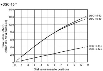
Note: Flow characteristics will vary based on pipe conditions and temperature changes before and after, and therefore caution is advised.
