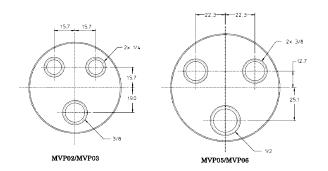
MVPO2 and MVPO3 models have 1/4" and 3/8" porting. MVPO5 and MVPO6 models have 3/8" and 1/2" porting. Imperial models are NPT thread and metric models are BSP thread.
