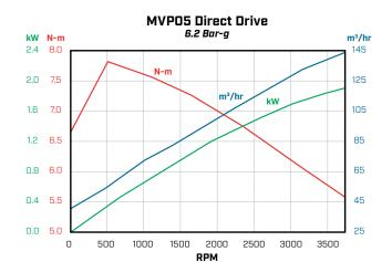
Example of the MVPO5 direct-drive air motor performance curve. See individual catalog pages for model-specific performance data.
