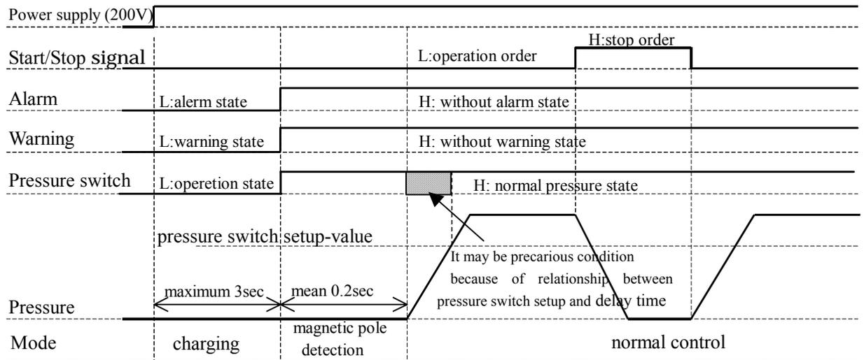
1-3 With using pressure switch function (Stopping when start power supply)
