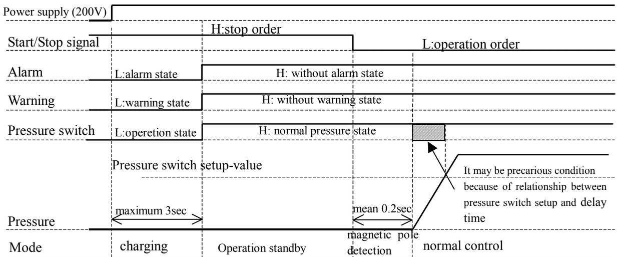
Magnetic pole detection is performed when first starting of motor.
