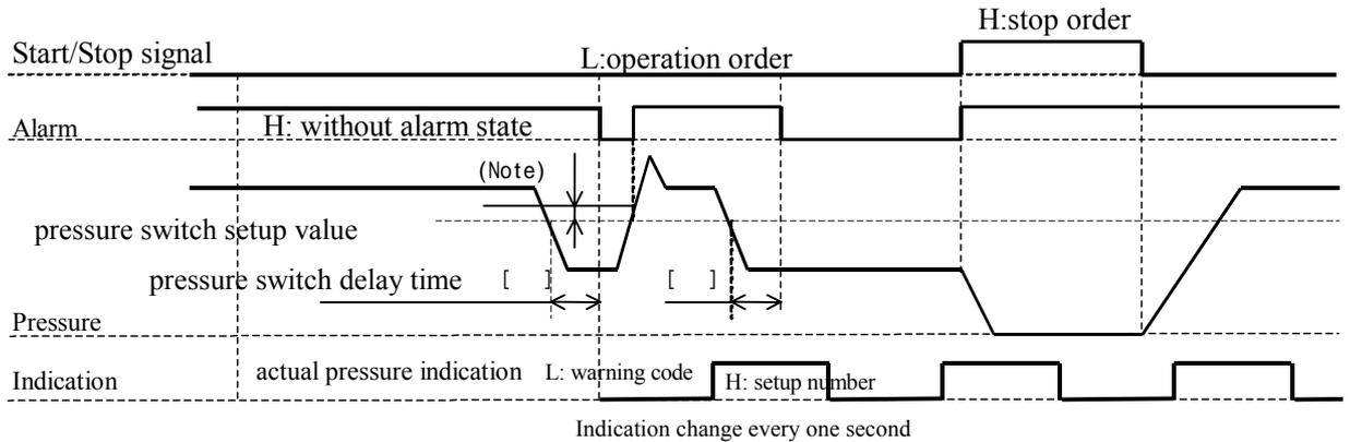
Above mentioned condition show when “08” (Indication hold setup of pressure switch) is [1] or [2].
