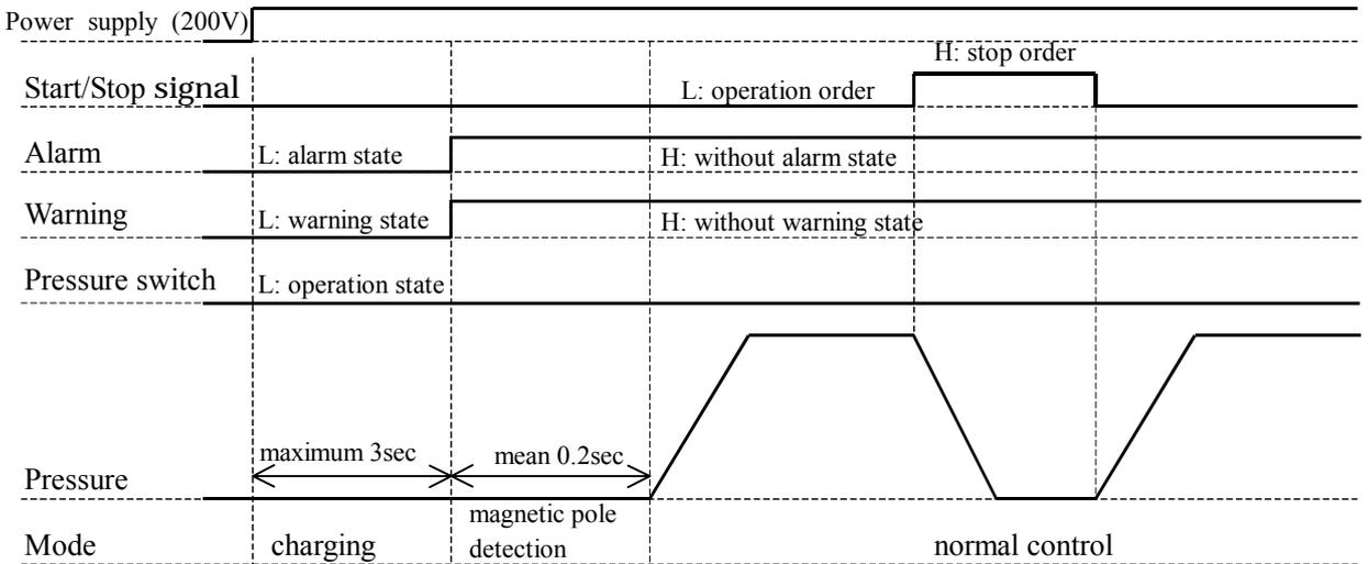
1-2 With using pressure switch function
