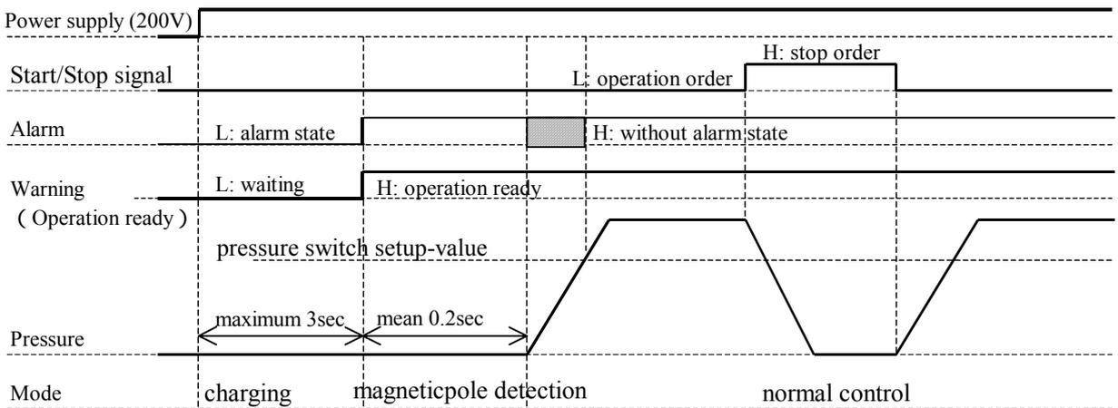
It may be precarious condition because of relationship between pressure switch setup and delay time.
