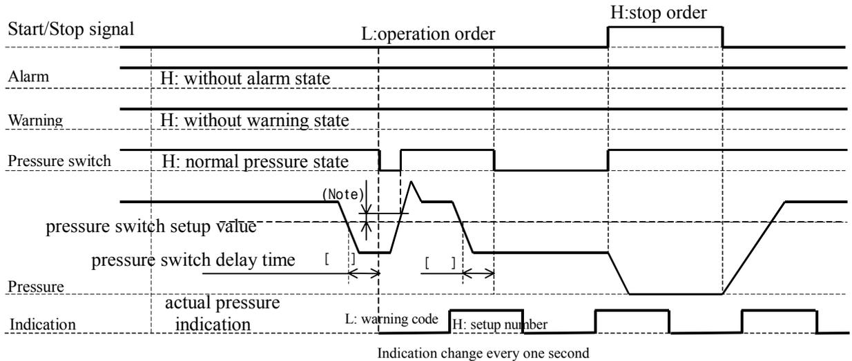
Above mentioned condition show when “08” (Indication hold setup of pressure switch) is [1] or [2].
