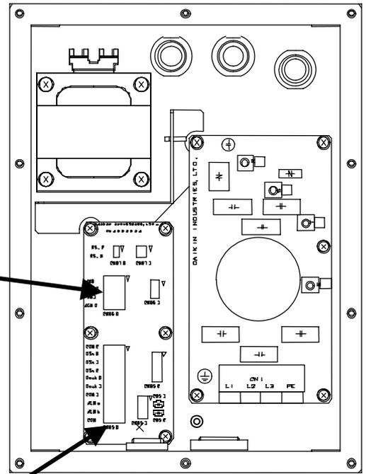
Input/output signal wiring diagram Terminal stand for alarm/control signal
