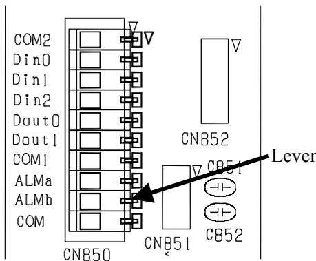
How to connect to the terminal stand board
