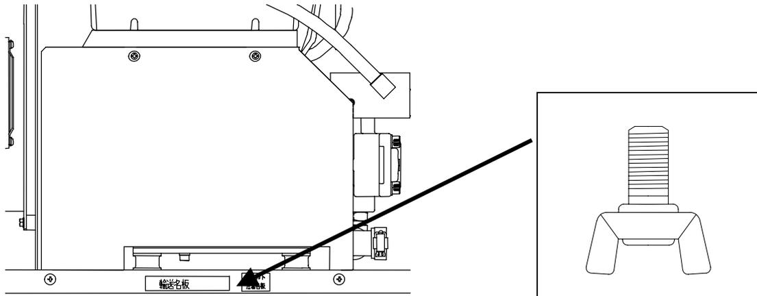
Wing bolt for fixing
