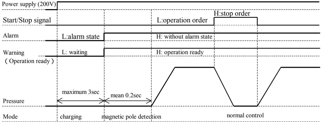
2-2 With using pressure switch function
