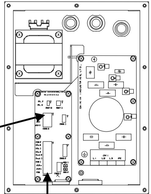
Terminal stand for alarm/control signal
