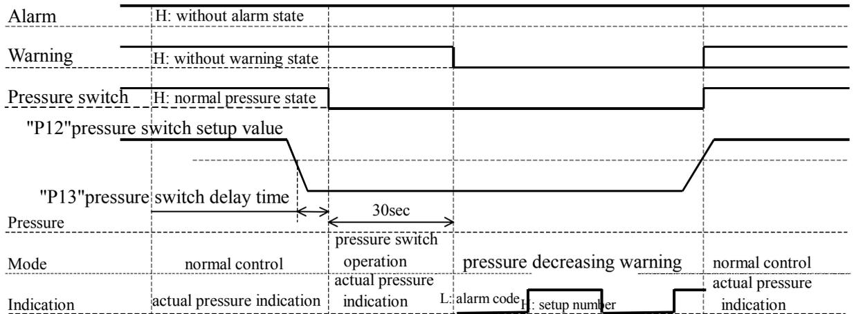
While holding pressure switch operation indication warning code and actual pressure are indicated by turns
