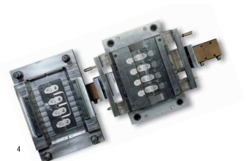
Production moulds are manufactured using modern CNC machine-tools.
