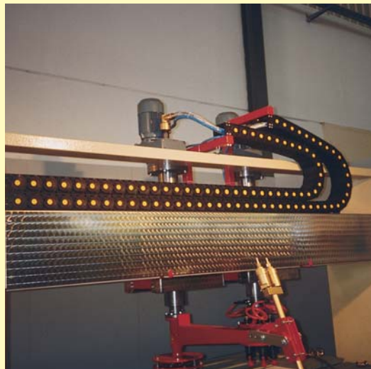
Model SR700 chains in nylon superimposed on a machine which works with marble.
