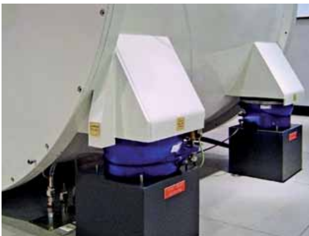
A measuring machine as an example of receiver isolation
