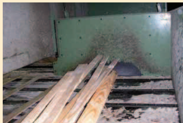
Impact protection for wooden battens
