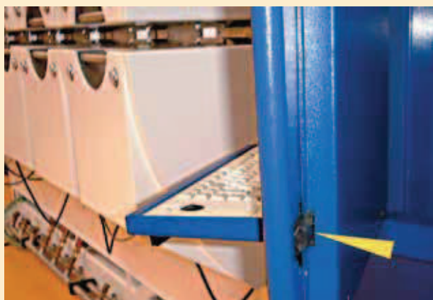
Pivoted machine keyboard
