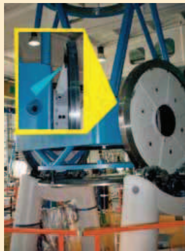
Perfect overshoot protection for precision telescope
