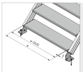
The depth of a step is determined by the Step Profile that is used. In the case of stairways with pitches of 30° or 38°, two Step Profiles 8 160 should be connected together using Step Profile Bracket Set 8 320. Step Profile 8 240 is ideal for 45° stairways. TPS enables users to build steps up to 1200 mm wide. The two 5 mm-wide fastening brackets must be taken into account when calculating the overall width.
