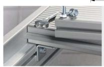
The Angle Bracket 8 and Step Spacer Profile, which is inserted into the groove between two panels in a platform, enable users to create an unbroken surface. Platform Cleats produce a 10 mm-wide gap between the panels in a platform.
