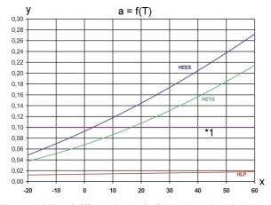
Water solubility of different hydraulic fluids determined by the temperature.
