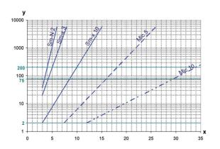
y = beta-value x = particle size [µm] determined by multipass tests (ISO 16889) calibration according to ISO 11171 (NIST)
