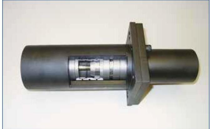
Schnittmodell Industriepuffer / Cross section of industrial buffer
