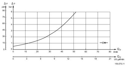
The check valve in the LS line of OSPC LS, OSPD LS and OSPQ LS dynamic steering units also protects the driver against steering wheel jerks. The check valve prevents oil from flowing backwards into the LS line to the priority valve when steering against a high pressure on the cylinder side.
