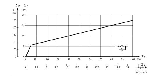
The curve below shows pressure drop for backpressure valve with by-pass.
